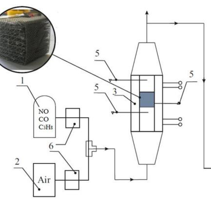
The total flow was 1.85 l/min per cartridge of catalyst.
