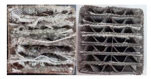
The geometry of structured elements doesn't appear to significantly affect the catalytic activity of CO and propane oxidation but produces definite difference in NOx reduction rate, with higher reduction activity for cartridges with volume metal mesh.
