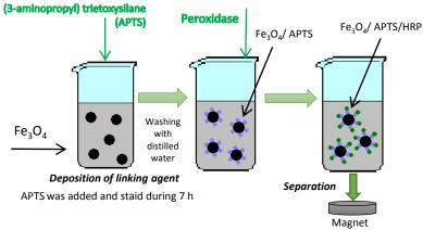
Scheme of the structure of the biocatalyst on the basis of HRP immobilized on MNPs
