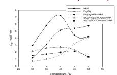
The increase of temperature higher than 40°C does not result in the decrease of activity in the case of the HRP immobilized on Fe<sub>3</sub>O<sub>4</sub> magnetic nanoparticles in contrast to the native HRP. The enzyme becomes thermostable. This is likely due to the strong binding of the HRP molecule with the support, which results to the stabilization of the enzyme conformation.
