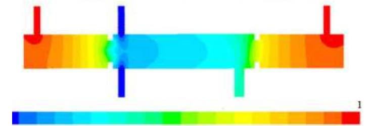
Figure 4 The methane mole fraction distribution in the longitudinal section (see online version for colours)
