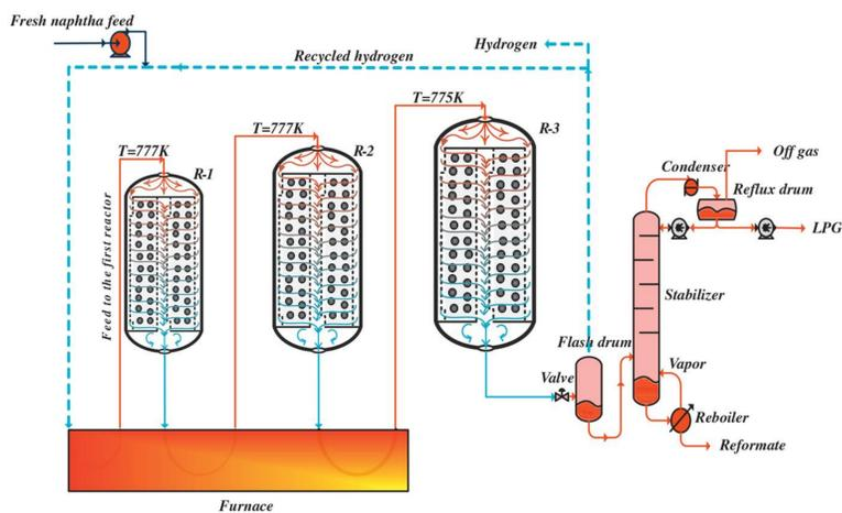
Schematic diagram of semiregenerative reforming unit with fixed-bed reactors [1]
