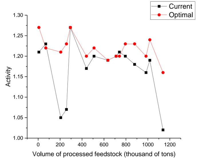
Comparison between current and optimal activity of catalyst (model calculation results)
