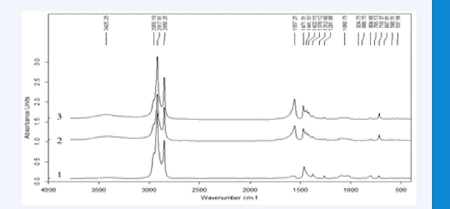
IR spectrum of  $\beta$ -sitosterol isolated from the original pine bark (1) and its activation products (2, 3): 2 - activation by explosive autohydrolysis under the following conditions: 120 °C, time 30 s, water vapor pressure 1.0 MPa; 3 - activation in a drum mill for 1 hour.
