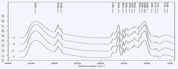
IR spectra of pine bark before (1) and after explosive autohydrolysis at different pressures (2 - 4): explosive autohydrolysis temperature 120 °C, time 30 s. 2 - pressure 1.0 MPa; 3 - 1.5 MPa; 1 - 2.0 MPa.
